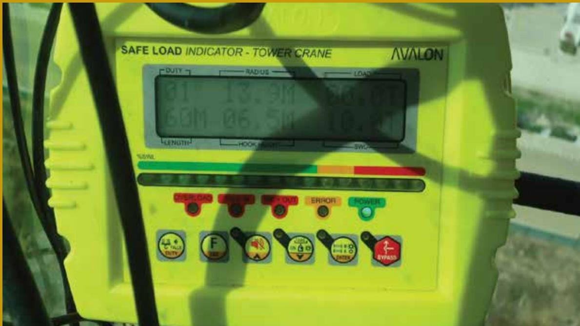
To ensure safety at site L&T's building factories business has installed Safe Load indicator on its tower cranes being used at its major projects.
