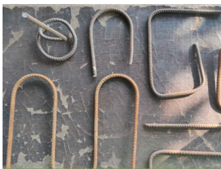
Scrap rebar used for structural work components
