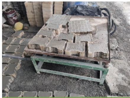
Paver blocks from recycled concrete waste
